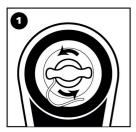
Release the valve cover by twisting counter - clockwise. Ensure the valve is clear from debris sand, or dirt before releasing.
