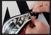
2 - Place the plastic washer, the steel washer and the M5x 29mm screw (in this sequence) in the preferred hole position.
