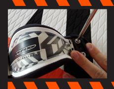
3 - It is IMPERATIVE to insert the screws along the vertical line of the insert hole. If you force the screw inside the hole you will permanently damage the board!
