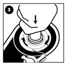
Insert the pump hose and twist it 45 degrees clockwise to lock in place. Inflate until you reach the required pressure 18 PSI
