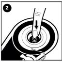
Push valve button in to lock it in **DOWN** position to deflate.
