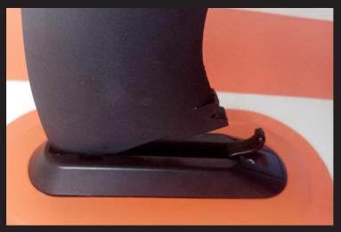
Open the click lever box and place the base of the fin in the plastic slot.
