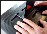
3 - Turn your assembled foil over and place it on your board above the US boxes. Use the 4 screws (and washers) to fix the foil plate to your board.
